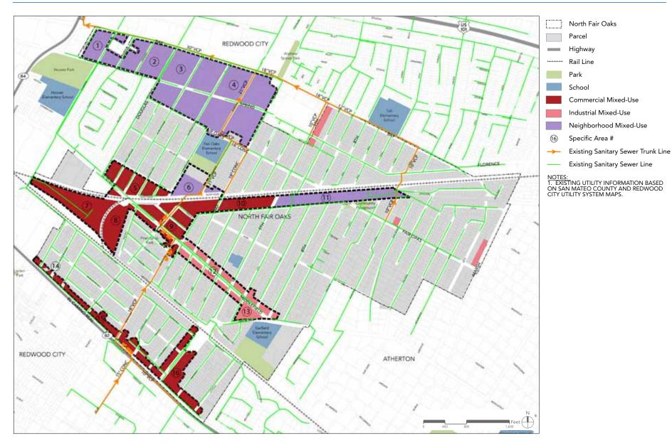
FIGURE 4.5: Proposed Sanitary Sewer System Improvements
